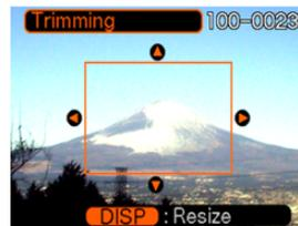
6. Use [**▲**], [**▼**], [**◀**], and [**▶**] to move the cropping boundary up, down, left, or right until the area of the image you want to extract is within the boundary.
