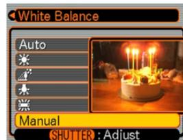
4. Point the camera at a white piece of paper or similar object under the lighting conditions for which you want to set the white balance, and then press the shutter release button.
