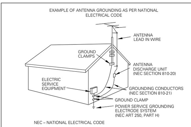
**18. Power lines** – An outside antenna system should not be located in the vicinity of overhead power lines or other electric light or power circuits, or where it can fall into such power lines or circuits. When installing an outside antenna system, extreme care should be taken to keep from touching such power lines or circuits as contact with them might be fatal.
