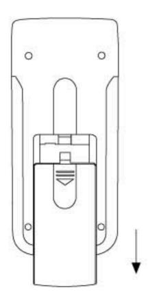
Insert two AAA batteries, make sure to match "+" and "-" on the batteries to marks inside the battery compartment.
