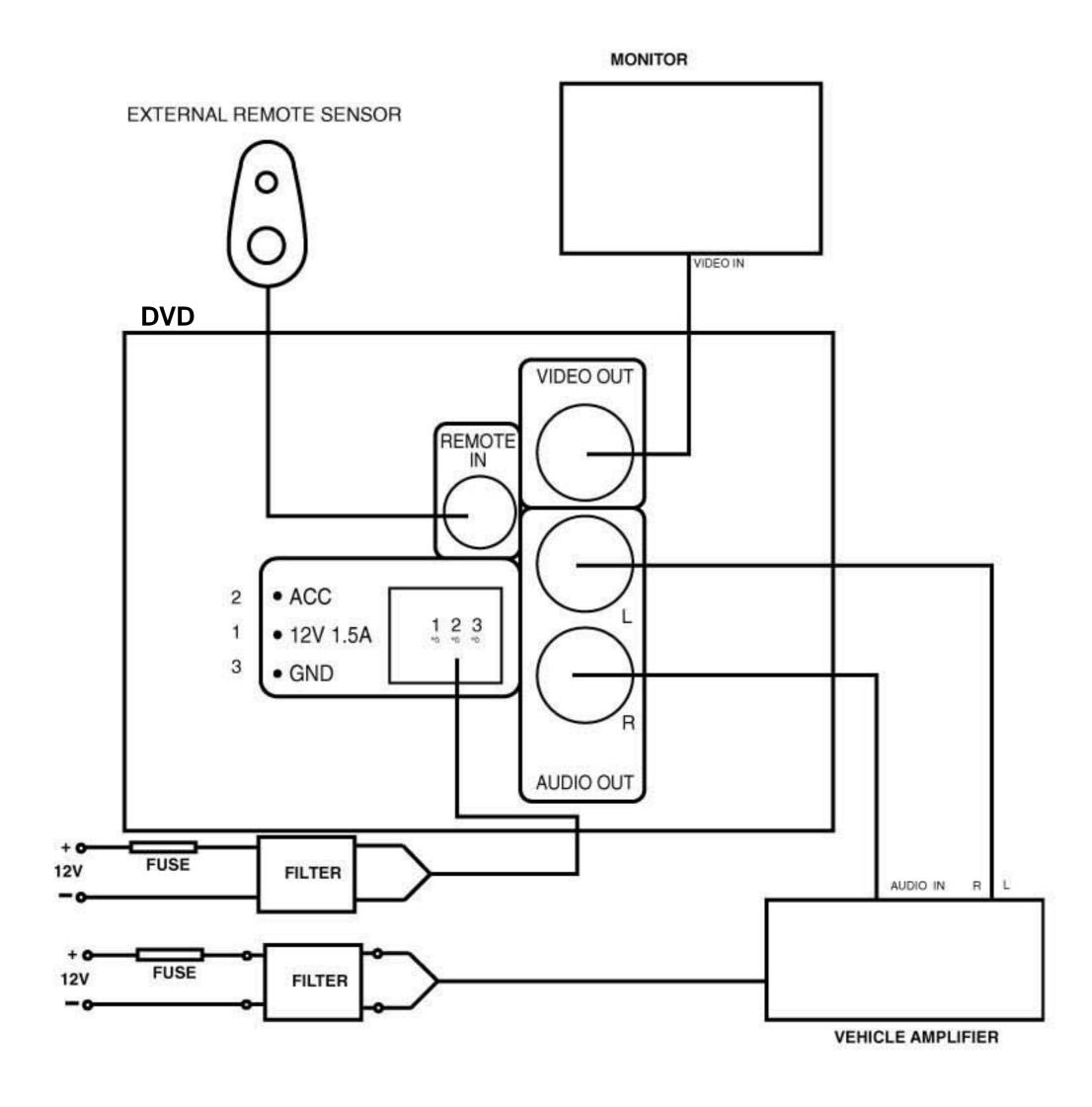
In the connection diagram above, the two "+" polarities can be simultaneously connected to the "+" polarity of the mobile DC 12V. And the two "-" polarities can be simultaneously connected to the "-" polarity of the mobile DC 12V.
