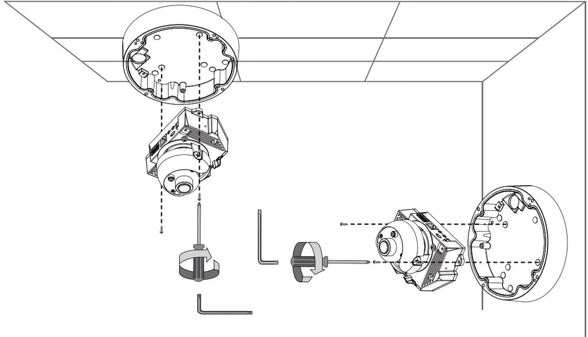
**Step 6** Feed a shielded twisted pair (STP) Category 5 or higher network cable through the conduit base and connect to the LAN port on the back of the camera. Connect the other end of the network cable to a 10/100/BaseT router or switch.
