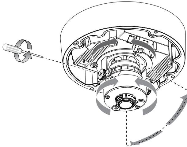
**Step 11** After you have adjusted the field of view, focal length, and zoom factor, install the black cover. Make sure to adjust it so that it does not block the lens from capturing video.
