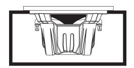
Box is given as internal air volume including driver displacement
