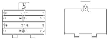
Press the battery door back on to the hinges, close the door, and rotate the locking tab back to the 6:00 o'clock position.
