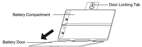
Insert 8 "AA" alkaline batteries in the compartment. Be sure to insert the batteries according to the polarity markings inside the compartment. If the batteries are inserted incorrectly the unit will not work.
