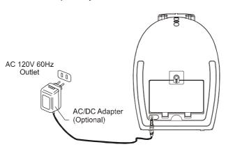
**Note:** When the AC adapter is connected to the back of the radio the batteries are automatically disconnected. You must disconnect the AC adapter from the back of the radio in order to operate the radio on batteries.
