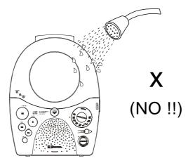
• When using the radio inside the shower use battery power only. Do not connect an AC adapter (not included).
