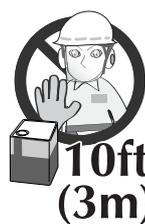
1. Always use caution when handling fuel. Wipe up all spills and then move the chain saw at least 10 ft(3 m) from the fueling point before starting the engine.
