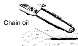
The chain oil flow can be changed by inserting a screwdriver in the hole on bottom of the clutch side. Adjust according to your work conditions.
