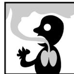
10. Operate the chain saw only in well ventilated areas. Never start or run the engine inside a closed room or building and potentially explosive atmosphere. Exhaust fumes contain dangerous carbon monoxide.
