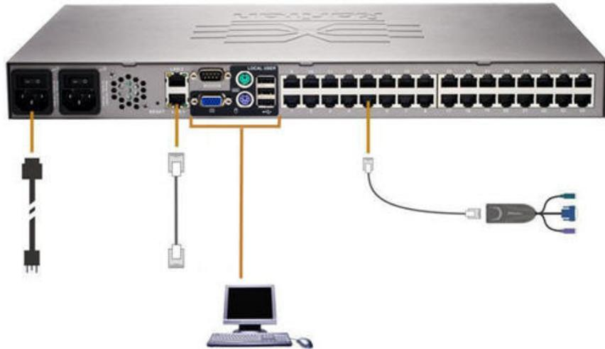
Figure 7: Dominion KX II Connections
