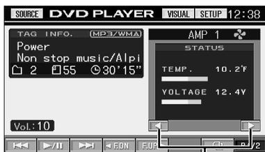
Changes the AMP display for the connected amplifier.
