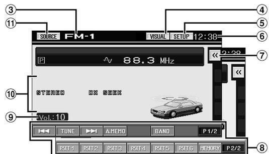
③ Displays the source name, such as radio band, etc., that is selected
