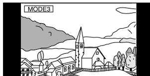
In Mode 3 (Normal), the monitor displays a normal picture at the center of the screen with a vertical black band at each side.
