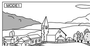
In Mode 1 (Wide), the monitor displays a normal picture wider to fit in a wide-screen monitor by evenly stretching out the picture horizontally.
