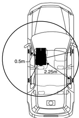
The sound is uneven because the distance between the listening position and the different speakers is different. The difference in the distance between the front left and rear right speakers is 1.75 meters (68-3/4").
