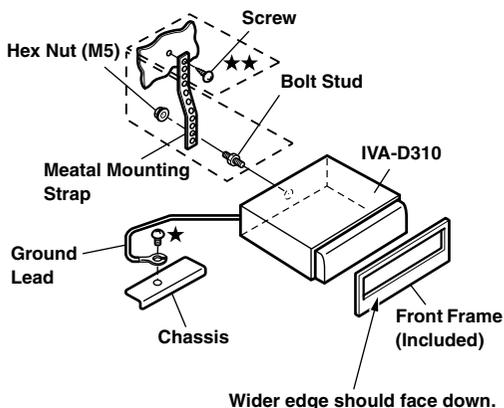
Reinforce the monitor unit with a metal mounting strap (not supplied). Secure the ground lead of the unit to a clean metal spot using a screw (★) already attached to the vehicle's chassis.
