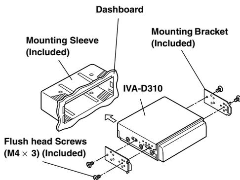
Slide the mounting sleeve into the dashboard. Install the supplied bracket on the monitor.
