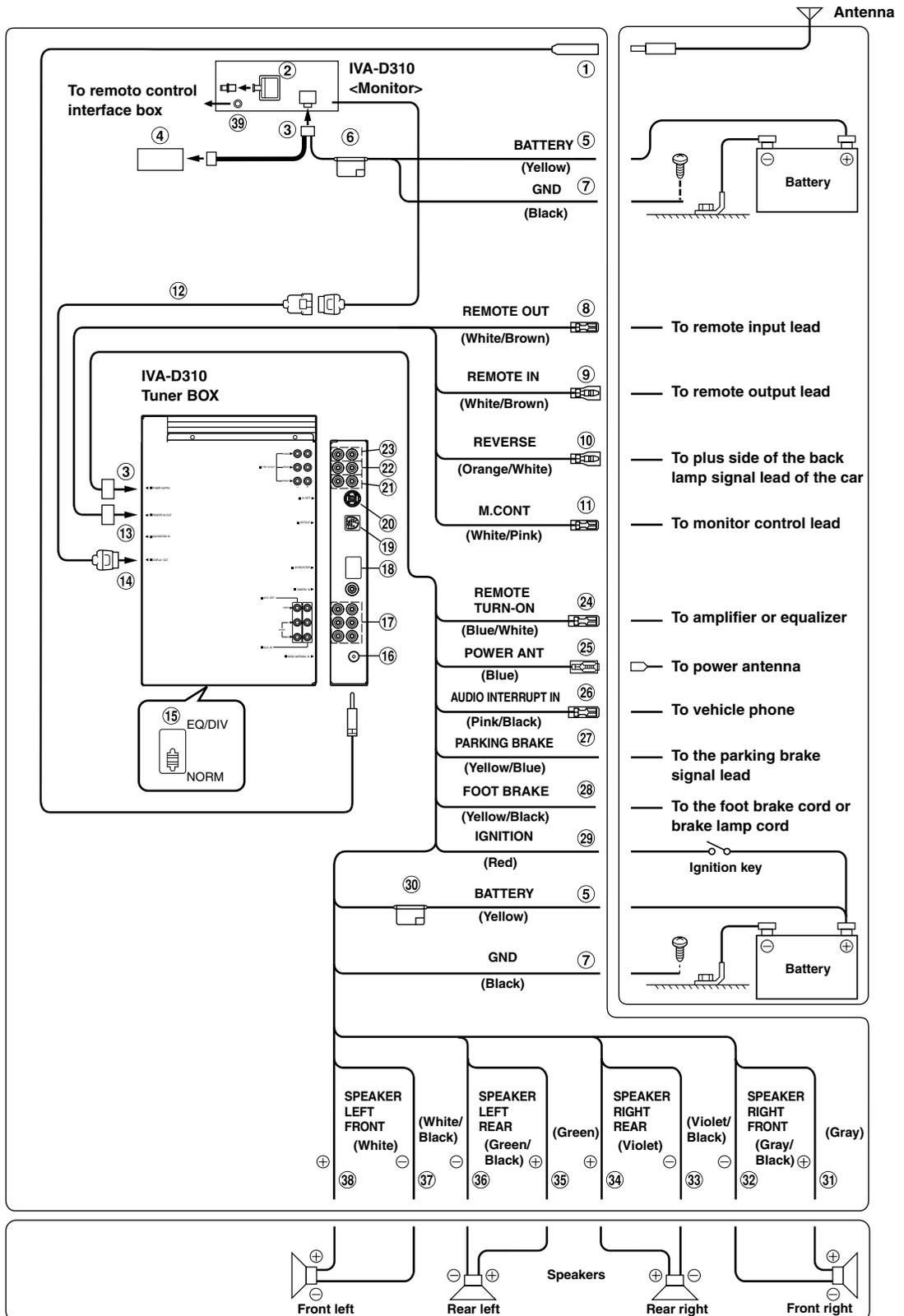
• Set the system switch to "NORM" when only a changer is connected (when the Ai-NET compatible equalizer is not used).
