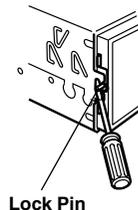
Slide the IVA-D310 into the dashboard. When the unit is in place, make sure the locking pins are fully seated in the down position. This can be done by pressing firmly in on the unit while pushing the locking pin down with a small screwdriver. This ensures that the unit is properly locked and will not accidentally come out from the dashboard. Install the supplied Front Frame.
