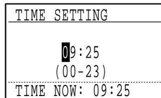
The current time appears in the screen. If the current time is not correct, press the [CA] key to cancel the operation and see "DATE & TIME SET" (page 104) to correct the time setting.
