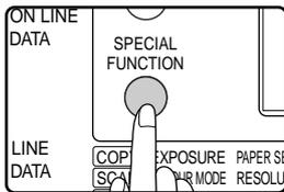
When the [SPECIAL FUNCTION] key is pressed, the special function selection screen appears. (To select fax mode, see step 1 on page 17.)
