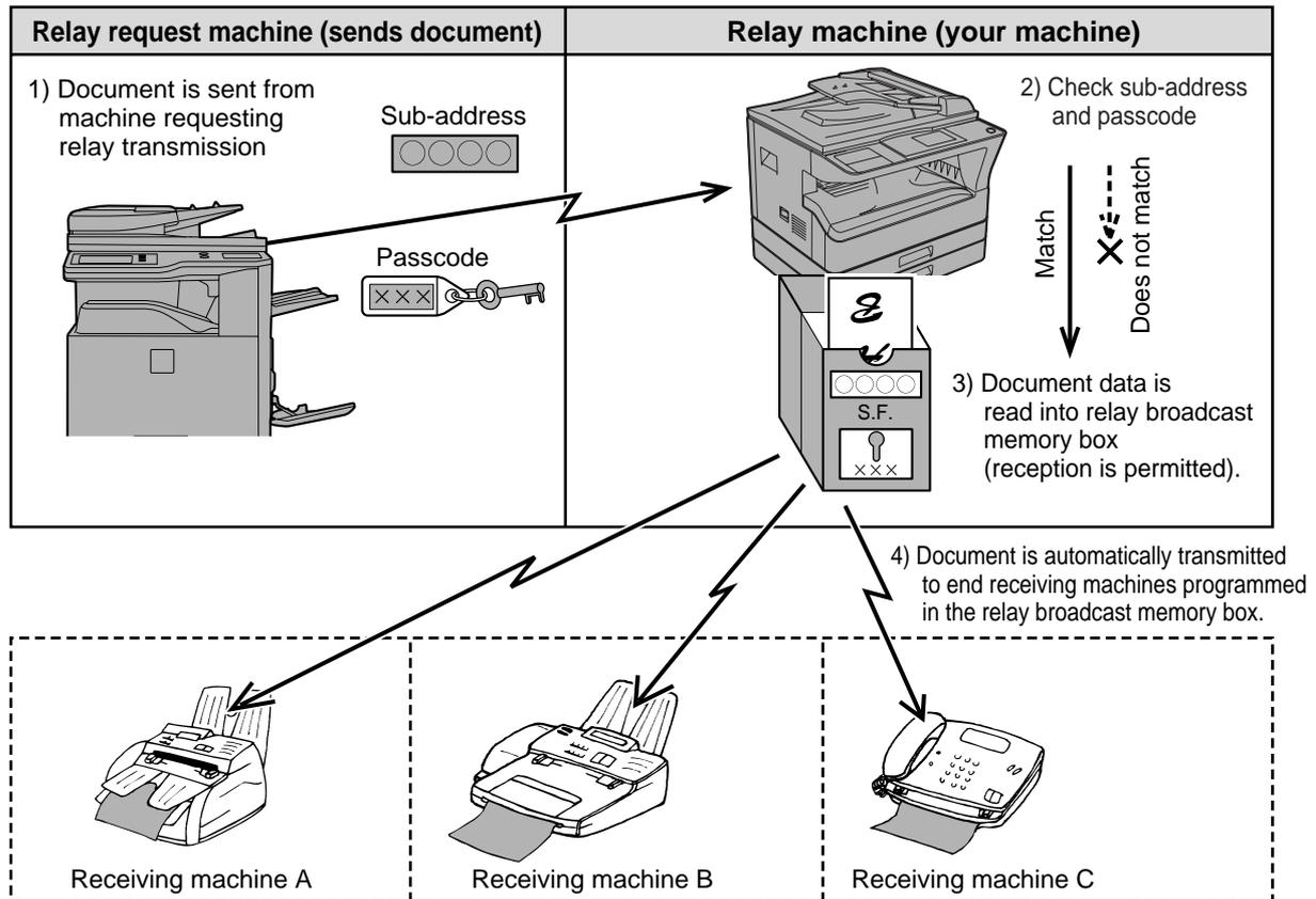
The machine that originally sends the document is called the relay request machine, and the machine that has a memory box containing the end receiving machines and which relays the received document to those machines is called the relay machine.
