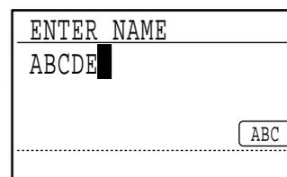
Up to 36 characters can be entered for the name. If you press the [OK] key without entering a name, go directly to step 13. In this case, a destination name will be assigned automatically.
