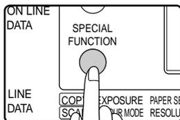
Press the [SPECIAL FUNCTION] key to display the special function menu. (To select fax mode, see step 1 on page 17.)
