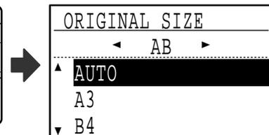
When the [ORIGINAL SIZE] key is pressed, the size selection screen appears. See "MANUALLY SETTING THE SCANNING SIZE" (page 13) to set the original size.
