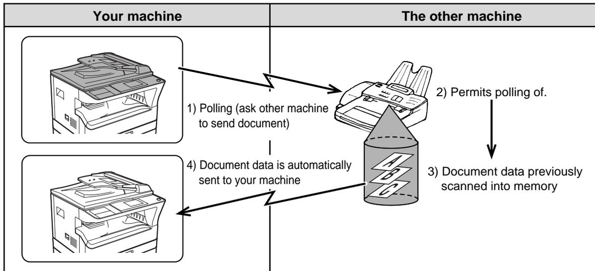
Group keys and the broadcast transmission function (page 31) can be used to successively poll multiple fax machines in a single operation (this is called "serial polling"). Up to 200 machines can be polled. In this case, the sequence of operations in the above diagram is successively repeated for each sending machine selected.
