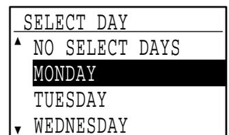
The selected day is highlighted. If you select "NO SELECT DAYS", the transmission will be performed as soon as the specified time arrives. To return to the [TIME SETTING] display, press the [BACK] key.
