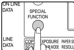
When the [SPECIAL FUNCTION] key is pressed, the function menu screen appears. (To select fax mode, see step 1 on page 17.)
