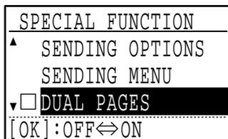
Dual Page Scan is selected when a checkmark appears in the "DUAL PAGES" checkbox. To cancel the selection when a checkmark appears, press the [OK] key in the next step so that a checkmark does not appear.
