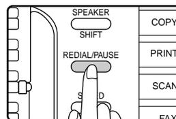
If a pause is necessary when dialling out from a PBX or when dialling an international number, press the [REDIAL] key. (This key functions as a pause key when entering a number.)
