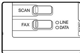
When the machine is in fax mode, the FAX indicator is lit. If the light is not on, press the [FAX] key.
