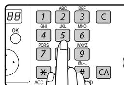
• Enter the 3-digit Speed Dial number entered when the Speed Dial number was programmed. (See step 7 of "Storing Rapid keys and Speed Dial numbers" on page 67.)
