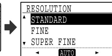
To adjust the resolution and exposure settings, press the [RESOLUTION] key. (See "SELECTING RESOLUTION AND EXPOSURE SETTINGS" on page 14.)
