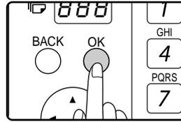
After entering a full number with the numeric keys, press the [OK] key to complete the entry. If you pressed an auto-dial key in step 3, it is not necessary to press the [OK] key. You can immediately press another auto-dial key for the next destination. Repeat steps 3 and 4 to select the remaining destinations.
