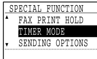
If a time has been specified, a checkmark appears in front of "TIMER MODE". To cancel a specified time, press the [\*] key in the above display with "TIMER MODE" highlighted.
