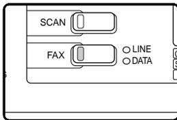
When the machine is in fax mode, the [FAX] key indicator is lit. If the indicator is not on, press the [FAX] key. If auditing mode has been enabled for the fax function in the system settings, a message will appear prompting
