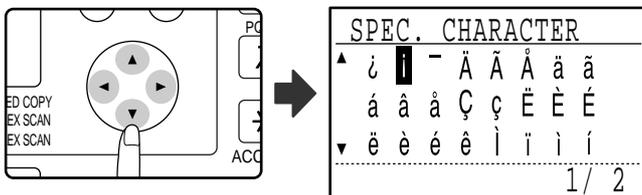
To move to the next page, move the cursor to the bottom line and press the [▼] key. To move back to the previous page, move the cursor to the top line and press the [▲] key. You can also change pages by pressing the [▶] key when the cursor is at the right end of the bottom line, or the [◀] key when the cursor is at the left end of the top line.
