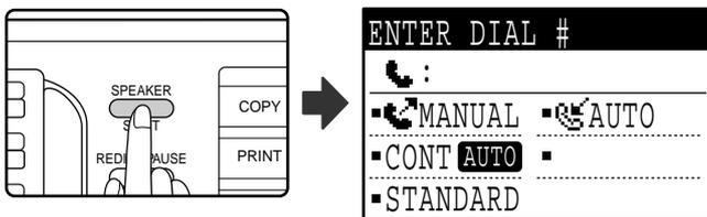
When this key is pressed, a message regarding volume adjustment will appear briefly followed by the dial entry screen. You can adjust the speaker volume (high, middle, or low) by pressing the [▼] or [▲] key. Note that this will not change the volume setting in the system settings. Ringing will be heard from the speaker on the left side of the machine (toward the back) when the [SPEAKER] key is used for dialling.
