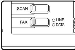
The FAX indicator is lit when the machine is in fax mode. If the indicator is not lit, press the [FAX] key. If auditing mode has been enabled for the fax function in the system settings, a
