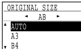
When the [ORIGINAL SIZE] key is pressed, the size selection screen appears. If the original size was not correctly detected, see "MANUALLY SETTING THE SCANNING SIZE" (page 13) and set the correct original size.
