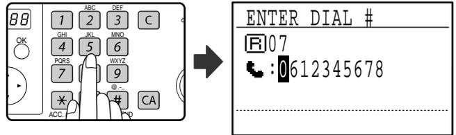
Move the cursor to the digit(s) that you wish to edit with the [◀] or [▶] key, and then enter the correct digit(s) with the numeric keys. To delete a digit, move the cursor to the digit that you wish to delete with the [◀] or [▶] key and then press the [C] key.
