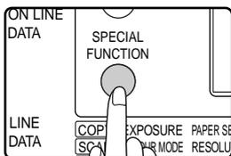
Press the [SPECIAL FUNCTION] key to display the special function menu.
