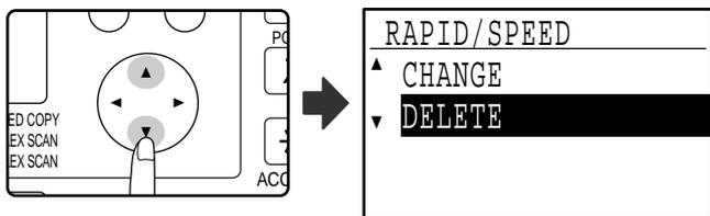
**2** Press a Rapid key ([01] to [50]) or the [SPEED] key.
