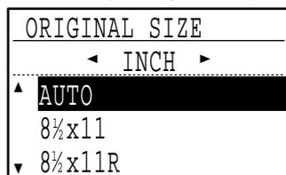
When the [▶] key is pressed, the original size selection screen for INCH sizes appears.
