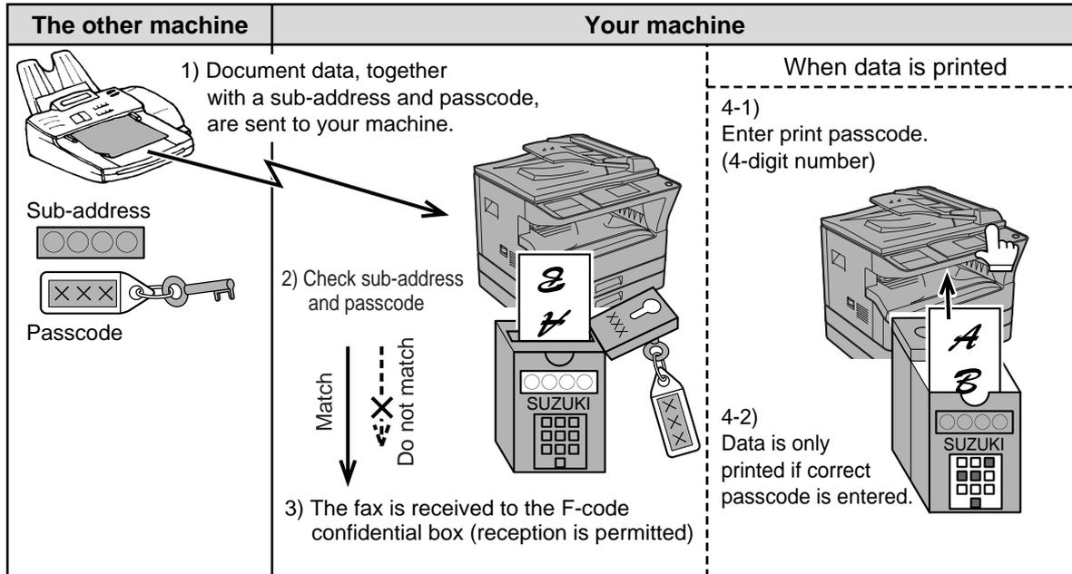
As the above diagram shows, receiving faxes to the machine's F-code confidential memory box is called F-code confidential reception, and sending faxes to another machine's F-code confidential memory box is called F-code confidential transmission.
