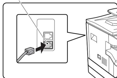
In some countries, an adapter is required to connect the telephone line cable to the wall telephone socket, as shown in the illustration.
