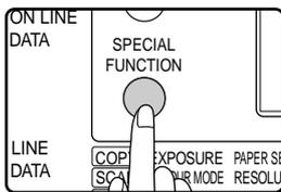
When the [SPECIAL FUNCTION] key is pressed, the special function menu appears. (To select fax mode, see step 1 on page 17.)
