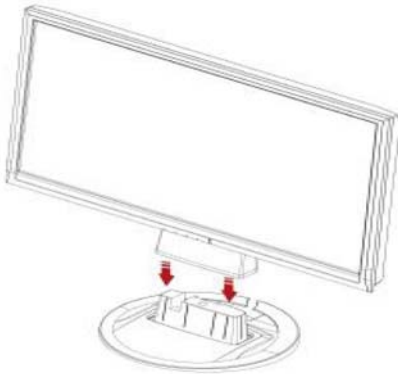
Figure.1. Installing and Removing the Base
