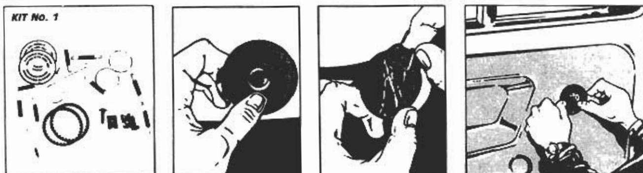
Place adhesive over pivot making sure that it adheres properly to door casing
