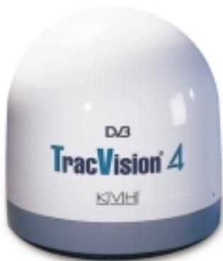
The Antenna Unit includes the antenna positioning mechanism, signal front end, power supply, and control elements. A molded ABS radome encloses the baseplate and is secured in place with flat head machine screws. Weathertight connectors located on the underside of the baseplate join the power, signal, and control cabling from below-decks units. A compression seal keeps moisture away from the connectors.
