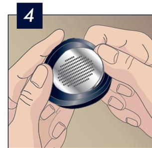
Remove the filter from the the gasket.
