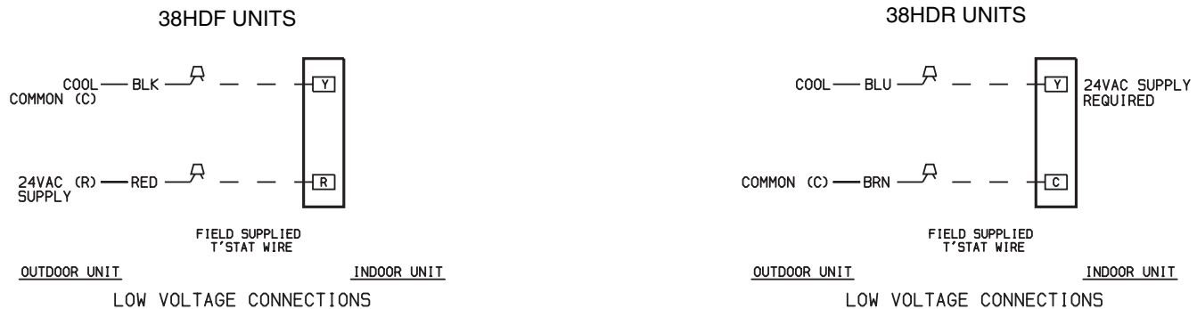
Fig. 5 — Typical Control Circuit Connections
