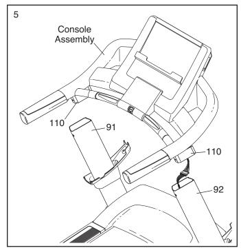
6. Partially tighten three 3/8" x 1 1/4" Patch Bolts (2) with three 3/8" Star Washers (6) into the Right Upright (92); do not fully tighten the Patch Bolts yet.
