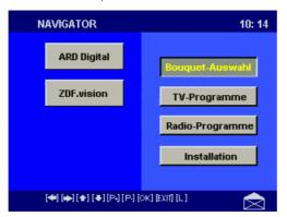
The name and time are displayed in the header line. The remote control keys that can be used for navigation are indicated in the footer line. If an open envelope is displayed in the bottom right-hand corner, a new software version can be loaded from the satellite (see "Initial settings", "Settings", "Software Update").
