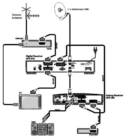
This configuration allows reception and VCR recording of digital programmes via the UFD 510 receiver as well as analogue, encrypted and unencrypted programmes via the secondary receiver (UFD 400 in this example).
