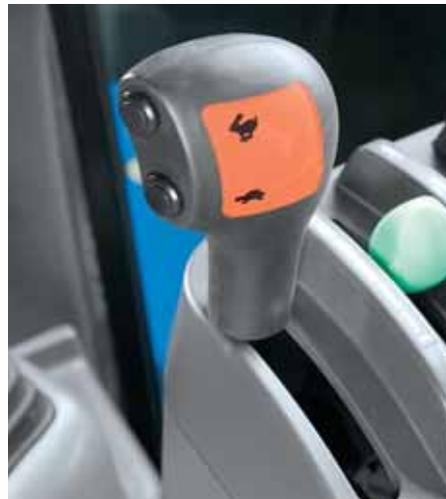
*The Hi-Low shift on the 24x6 synchronized transmission is integral with the throttle lever for easy operation.*
