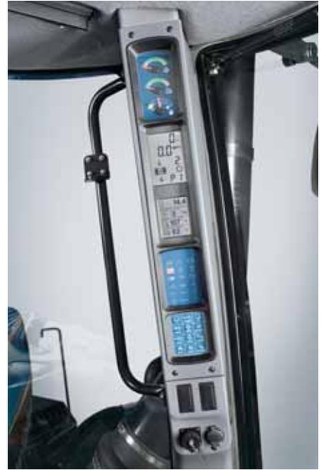
All the information you need on the go and at a glance — you can monitor everything from wheel slip and ground speed to fuel usage and hydraulic-flow readings with the optional performance instrumentation that's integrated into the cab post for easy viewing.
