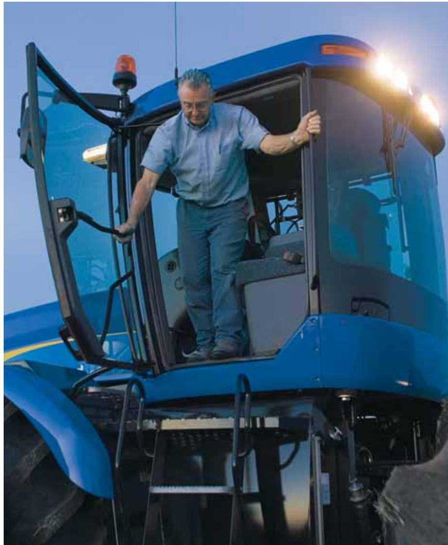
Convenient egress lighting lets you safely exit the cab while in a dark environment. Egress lighting is standard equipment on all T9000 models.
