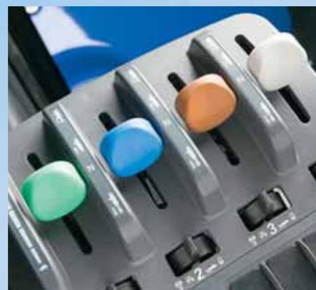
*Hydraulic control levers and couplers are color-coded for ease of hook-up and to help track hydraulic operations.*
