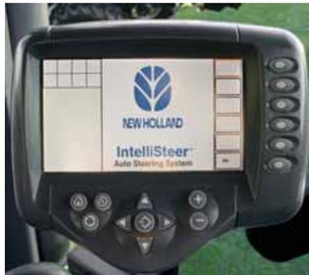
The New Holland VT™ colour monitor provides complete interface with the IntelliSteer™ system.
