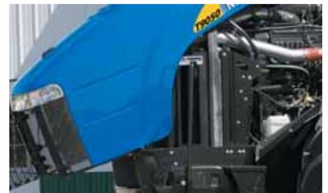
*The cooling system provides the extra cooling capacity needed with higher-horsepower engines. The radiator is sized to the engine and can be accessed easily for cleaning.*
