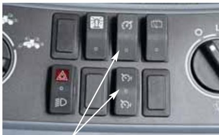
*Use the constant speed switches to set the max RPMs and the speed adjustment switch or throttle to return engine speed to the desired level after making a turn.*
