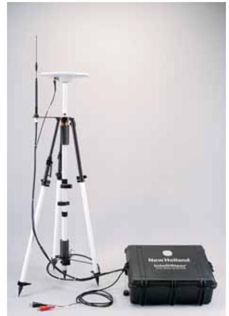
The RTK base station includes a GPS antenna, receiver and radio link to provide RTK correction signals to tractor-mounted auto-guidance systems and can be either portable or permanently mounted.
