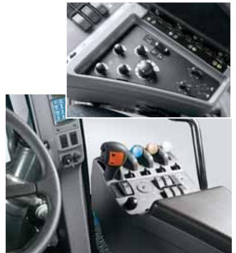
Right at hand . . . controls for AutoShift™ hydraulic remotes, flow and timer, diff lock, hitch, custom headland management, optional slip limit, throttle and gear selection are integrated into the armrest for ready, comfortable access.
