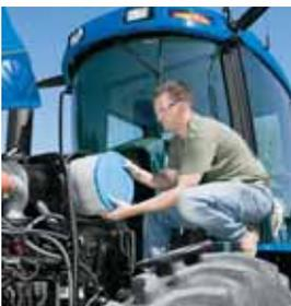
grill swings open for easy access to the radiator and cooling system. A radiator overflow bottle allows for quick visual checks of coolant level. And, a clean-out trap door located under the radiator, allows you to clean the radiator and cooling system without hassles.
