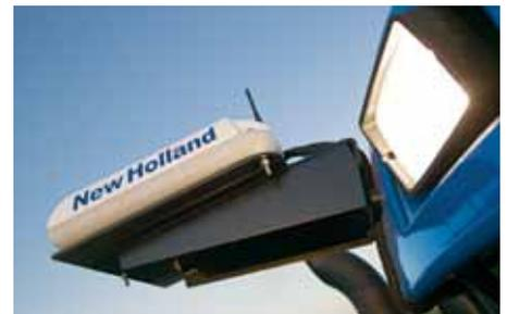
The New Holland 252 antenna receives the GPS signals to guide the vehicle. This antenna can easily be transferred from tractor to tractor or even to your combine.
