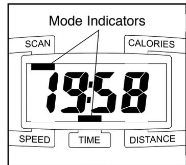
**Speed, time, distance, or calorie mode**—To select one of these modes for continuous display, repeatedly press the Mode button. The mode indicators will show which mode is selected. Make sure there is not a mode indicator below the word “SCAN.”
