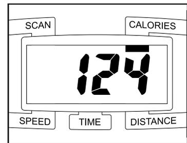
**Note: The console can display speed and distance in either miles or kilometers. To change the unit of measurement, press the On/Reset button for about five seconds.** The letters mph or km/h will appear in the display to show which unit of measurement is selected. When the batteries are replaced, it may be necessary to reselect the desired unit of measurement.
