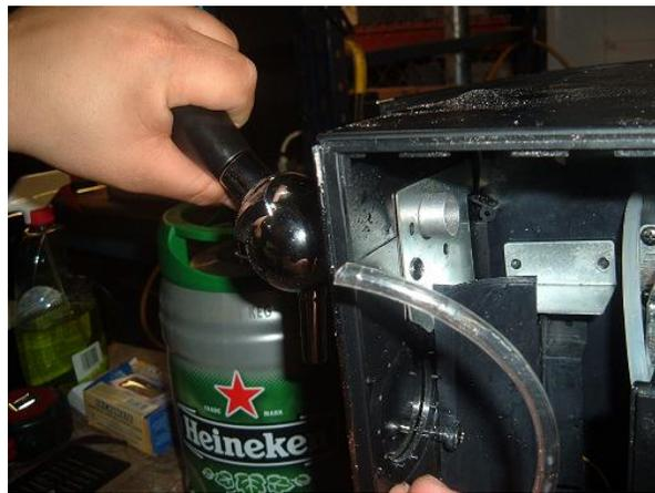
4.) Next, insert the new hose the same way you removed the old one. Pull and hold the lever down and insert the new hose from the back. Keep pushing the hose in until you can see it coming out the faucet. Then pull it back about 1/4 inch. Reattach the hose to the beer line and then screw on the coupler as pictured below and your done. Then put the side panel back on.
