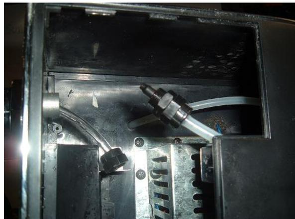
3.) Then, while pulling the tower lever down (as if opening to pour beer), pull the hose out from the back side as pictured below.
