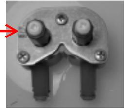
13. To disassemble the flow control: Remove screws and pull retainer forward. Remove top flow control subassemblies exposing flow controls. Note the difference between high flow and ultra flow valves.
