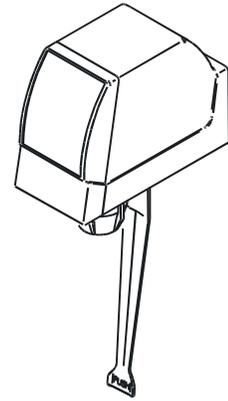
\*Note: A metal rivet in the valve body supplies electricity through the beverage being dispensed. When the foaming beverage comes in contact with the metal dispensing lever it completes the electrical circuit and the flow module closes the dispensing valve — even though the lever is still activated.
