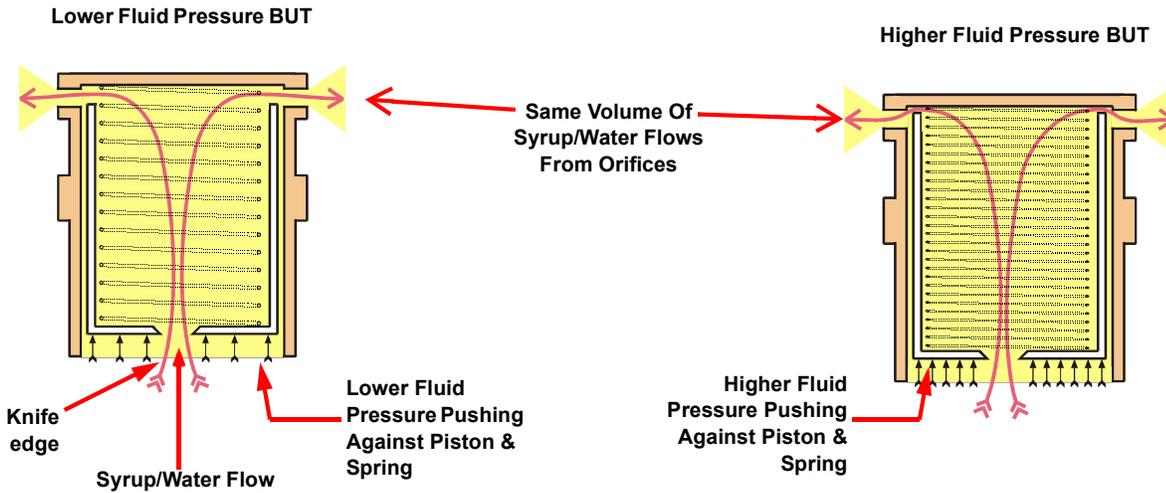
The position of the piston inside the sleeve is determined by the upward pressure of the liquid against the base of the piston and the downward pressure of the spring inside the piston (not shown here). The pressure of the spring is regulated by the adjusting screw.
