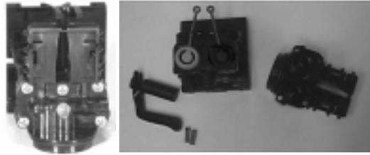
17. To remove the dispensing lever return spring pry the end of the spring and pull up. This spring stops the lever from vibrating.
