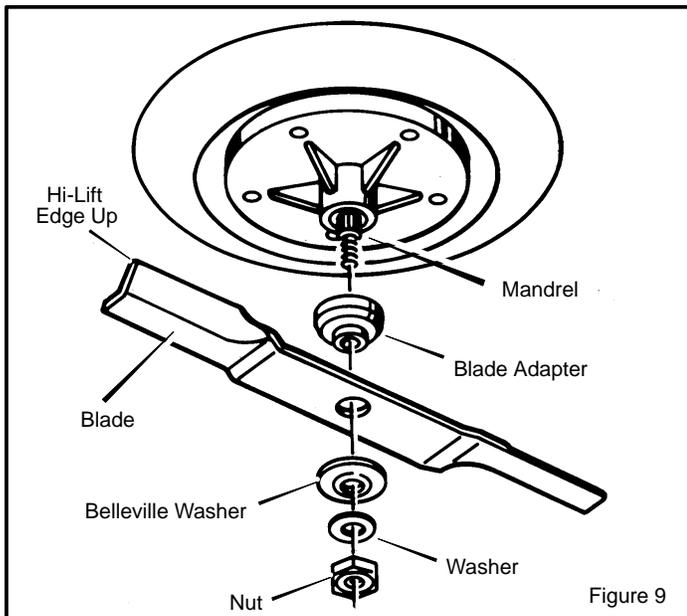
4. Check the **blade** and the **blade adapter** according to the instructions for "Inspect Blade". Replace a badly worn or damaged **blade** with an original equipment blade. See an authorized service center in your area.
