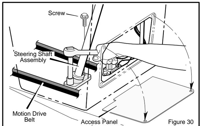
11. Remove the **motion drive belt**. A correct replacement part or assistance is available from an Authorized Service Center in your area.
