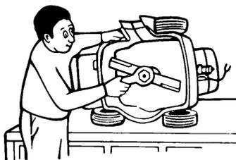
A sharp blade decreases the workload on the engine and more evenly cuts grass. Frequently sharpen the blade for a better looking cut. Use the left side of the mower housing to trim near an object.
