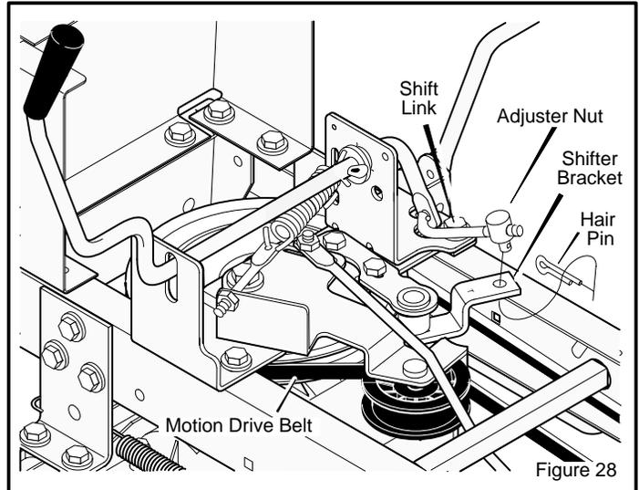
8. To remove the **motion drive belt** from the **stack pulley**, pull the front end of the belt under the **stack pulley** and then back between the stack pulley and the **steering plate** (Figure 29).
