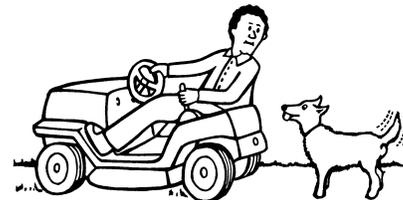
Before you leave the mower, stop the engine. Remove the key. Disengage and lower any attachment. Set the parking brake. Never mount or dismount from the seat while the engine is running. An accident can occur if you touch the brake, shift lever, throttle, clutch or blade control while the engine is running. Mount and dismount from the seat on the side of the unit that is marked ENTER-EXIT.
