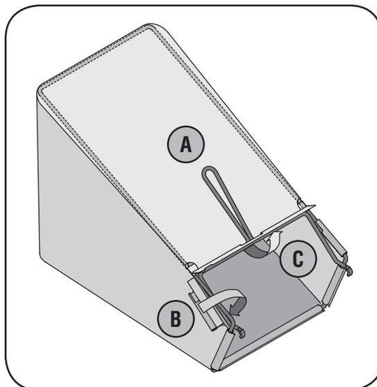
Figure 3-7: Assemble the grass catcher (if needed).
