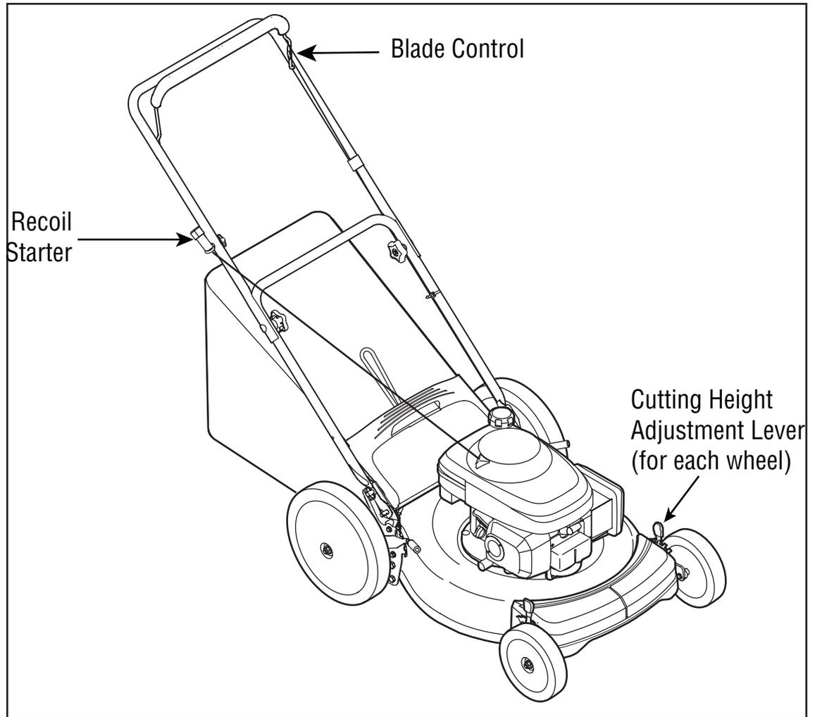
Figure 4-1: The main components on the mower.
