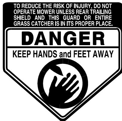
Figure 1 Safety Labels Found On Lawn Mower
