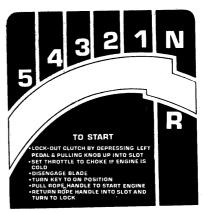
FIGURE 8. SHIFT PATTERN (Recoil)
