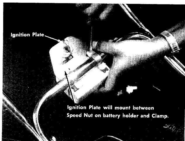
FIGURE 6. ASSEMBLY OF IGNITION PLATE
