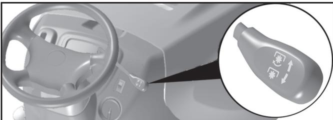
(\*) ATTACHMENT CLUTCH LEVER "DISENGAGED"
