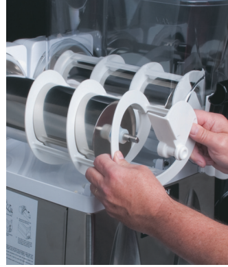
3. Align the auger shafts with the augers. Push the augers as far as they will go and rotate them so the flat face of the auger shaft is aligned with the flat face of the auger nose.
