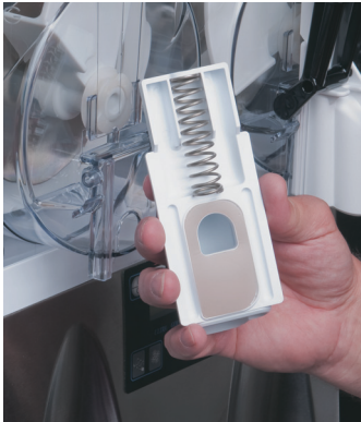
5. Position the faucet seal and the return spring in the faucet valve.
