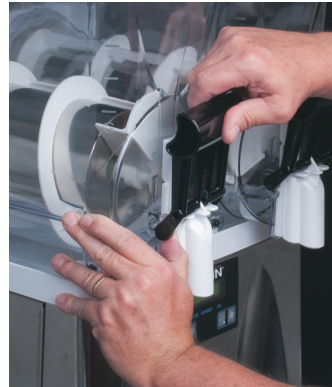
7. Press down on the valve to compress the spring. Position the faucet handle over the faucet valve one side at a time and snap into place on the hopper.
