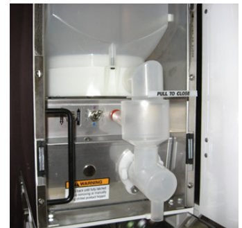
11. Reassemble and install all PAF parts. Return power switch to the ON position. Close Door.
