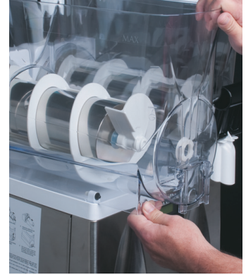
4. Install the hopper over the auger and cooling drum and slide it into place. Push down until the hopper lock plunger snaps into place .
