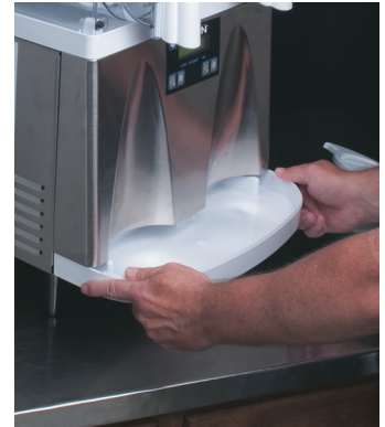
8. Install the drip tray and cover.
