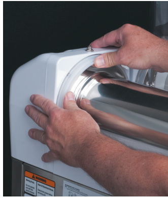
2. Install the hopper seal over the flange at the rear of the cooling drum as shown.
