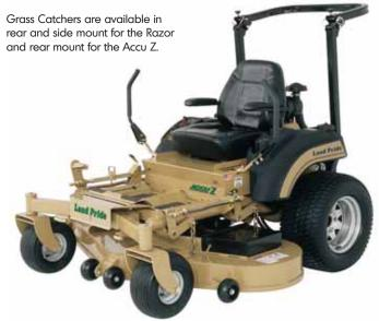
Optional ROPS is available for added operator protection. Available in fixed or folding for cutting under trees.
