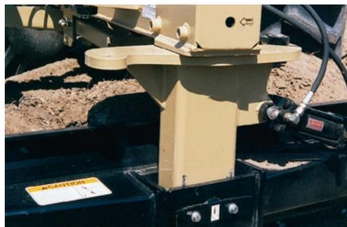
RBT45 features a 1" thick plate steel turntable, 3/8" thick tilt pivot bushing and a 4" solid kingpin.
