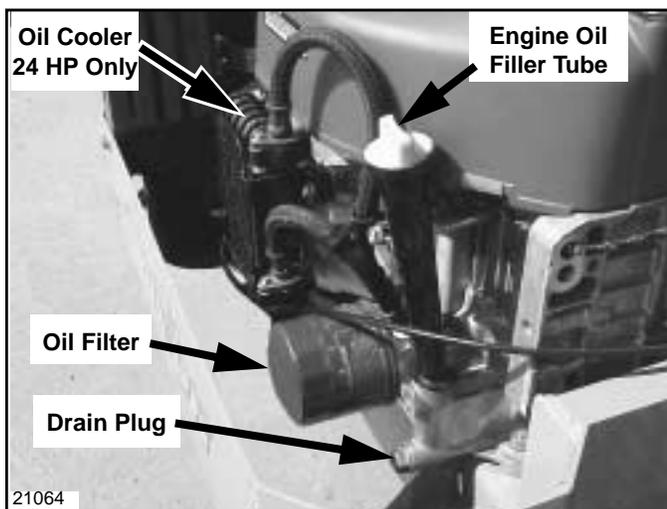
Honda Engine Oil Filter, Drain & Filler Tube
