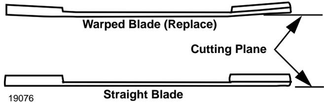
**Comparison of Warped and Straight Blades**
