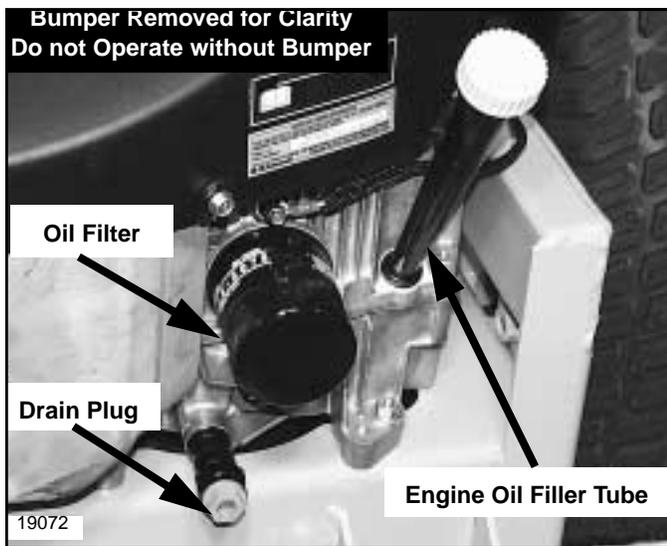
Kawasaki Engine Oil Filter, Drain & Filler Tube
