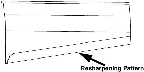
Do not sharpen to original pattern (below). It is easier to get a straight cutting edge following the resharpening pattern shown above.
