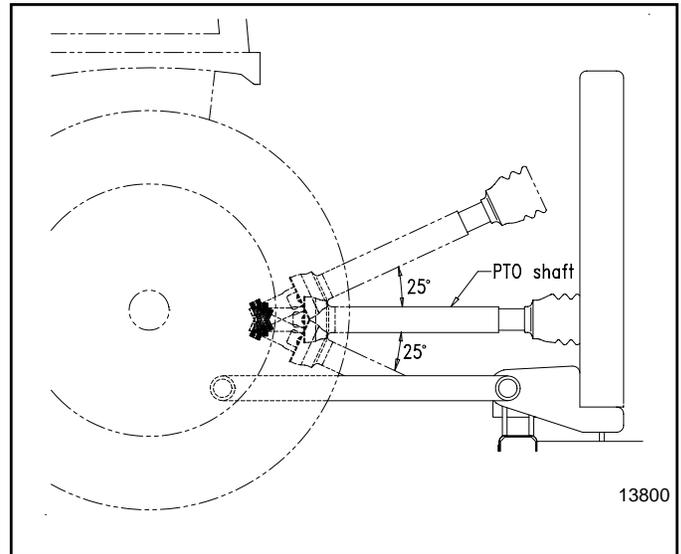
Maximum PTO driveline Movement During Operation
