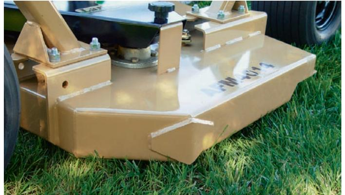
The front corners of each deck are reinforced to protect against hitting obstructions. Smooth outside deck construction saves trees and other obstructions.
