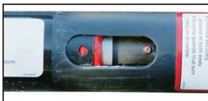
Easily access grease zerks to keep drivelines operating efficiently.
