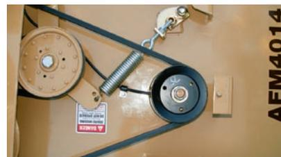
Over center release easily takes tension off the drive belts during extended off time.
