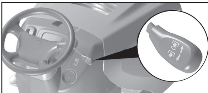
(☒) ATTACHMENT CLUTCH SWITCH "DISENGAGED"
