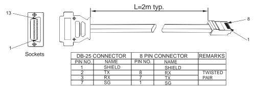
Fig.7-2: RS232 cable with DB25 connector (P/N: GEN/232-25)
