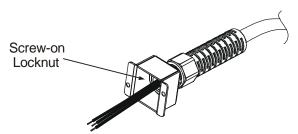
Fig.3-2: Stripped Wires installed in Strain Relief
