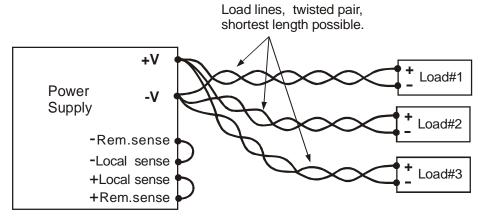
Fig.3-13: Multiple loads connection, radial distribution, local sense
