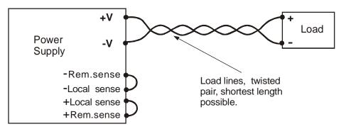
Fig.3-11: Single load connection, local sensing
