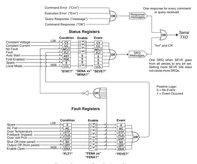
Fig.7-7: Status and Error Registers Diagram
