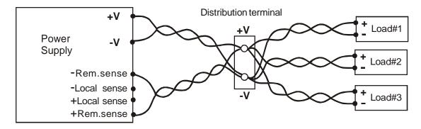
Fig.3-14: Multiple loads connection with distribution terminal
