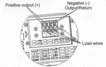
Fig.3-8: Load wires connection to the output connector
