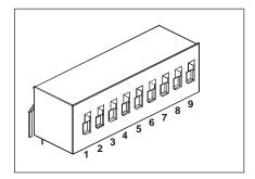
Fig.4-3: SW1 setup DIP-switch
