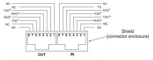
Fig.7-1: Rear panel J3 IN/OUT connectors pinout
