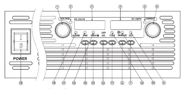
Fig.4-1: Front panel controls and indicators
