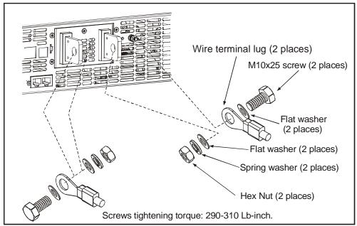
Fig. 3-6: Load wires connection, 8V to 100V models
