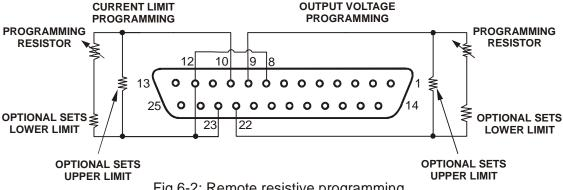
Fig.6-2: Remote resistive programming
