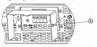
Fig.3-9: Shield assembly
