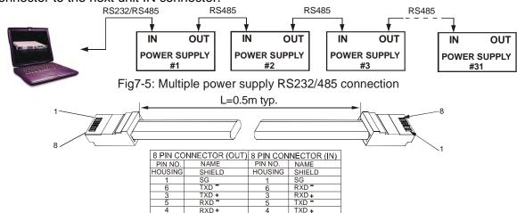
Fig.7-6: Serial link cable with RJ-45 shielded connectors (P/N: GEN/RJ-45)
