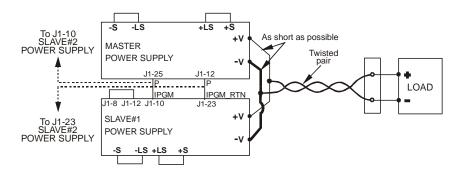
Fig.5-4: Parallel connection with local sensing
