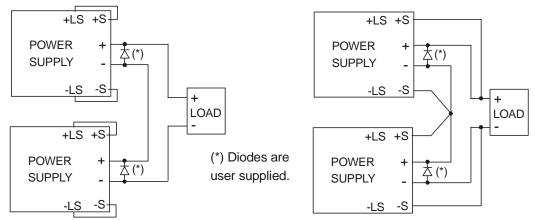
Fig.5-1: Series connection, local sensing
