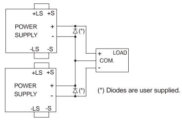
Fig.5-3: Series connection for positive/negative output voltages
