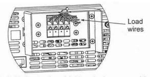
Fig.3-10: Protective shield and wires assembly
