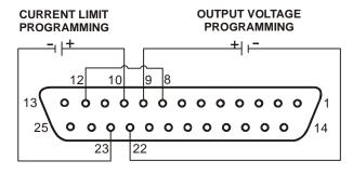
Fig.6-1: Remote voltage programming connection
