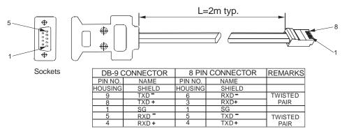
Fig.7-4: RS485 cable with DB9 connector (P/N: GEN/485-9)
