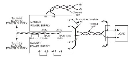
Fig.5-5: Parallel operation with Remote sensing
