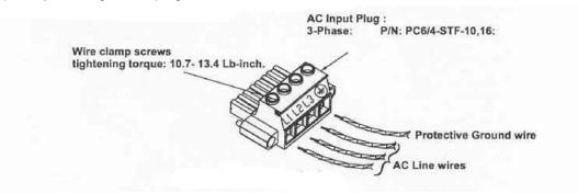
Fig.3-3: AC Input plug (3-Phase shown)
