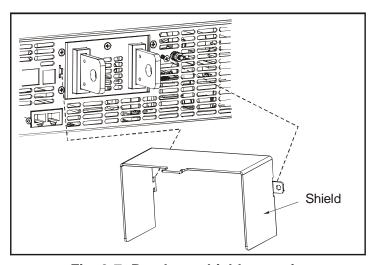
Fig. 3-7: Bus-bars shield mounting
