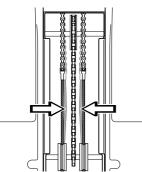
3 If necessary, the wires can be adjusted by tightening the adjuster nuts on each side of the steering collar. Do not over tighten the cables; they should only be drawn in towards the steering collar.
