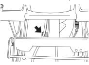
4 Push the unit in and put the guide plugs in the grooves on the equipment frame, one on each side.
