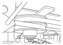
4 Reset the cutting unit from service position to mowing position.
