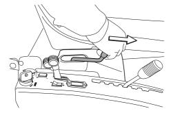
4 Select the required cutting height (1-7) with the cutting height lever.
