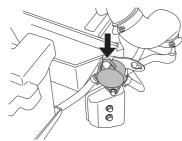
• Replace the pump on the console.
