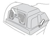
Cooling is impaired if the air intakes are blocked or the transmission housing is dirty, this can result in damage to the transmission.
