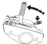
3 Remove the front hood by removing the pin. (There are complete instructions on using the service position inside the front hood).
