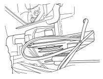
6 Fit the hose holder in the middle and the belt guide for the centre belt.
