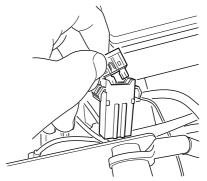
The fuse for the power outlet is placed under the ignition switch, behind the side plate on the control panel. Type: Flat pin, 7,5 A.
