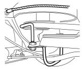
5 Pull off the centre belt from the engine's pulley and pull out the rear section.
