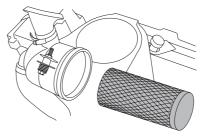
4 Clean the filter by knocking the filter carefully against a hard surface and blowing with compressed air from inside. Never brush the dirt away. Replace the air filter if it is very dirty.
