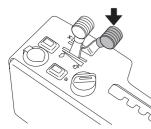
8 Let the engine run at moderate speed or half throttle for 3-5 minutes before subjecting it to heavy load.
