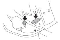
3 Press in the lock button on the mechanical lifting lever and lower the cutting unit.
