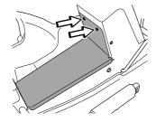
• Work the pedals and lubricate the moving parts with an oilcan. Lubricate the cables for the brake and drive pedals using an oil can.
