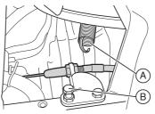
4 Remove the hose holder in the middle and the belt guide for the centre belt.
