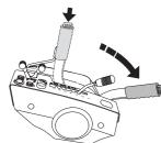
If this does not happen it is probably because the unit has been lifted with the hydraulic lifting lever. Lower the unit to the mowing position with the lever for the hydraulic lift.
