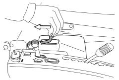
Secure the cutting unit if necessary using the mechanical lifting lever.
