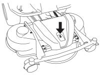
The front cover is secured to the unit frame with two hooks.
