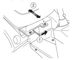
The seat springing can be adjusted by moving the rubber stops in their mountings on the underside of the seat. Place both stops in the front, middle or rear.
