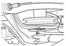
9 Pull out the belt through the opening under the pivot bearing and past the belt tensioner's disc.
