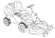
The machines are equipped with power steering and hydraulic lifts. PR 17 AWD and PF 21 AWD also have all wheel drive.
