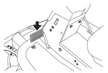
2 Carefully press down one of the pedals until the required speed is obtained. Pedal (1) is used to drive forwards, and pedal (2) to drive backwards.
