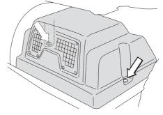
• Check that there is oil in the transmission's oil tank.
