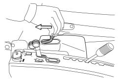
The unit can then be secured in the raised position if necessary by moving the mechanical lifting lever backwards to the lock position.
