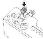
9 Set the required engine speed with the throttle control.
