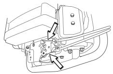
• Lubricate the joints, catches, and bearings for the cutting unit's control levers with an oilcan.
