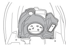
A blocked cooling intake will interfere with the cooling of the engine, which can damage the engine.
