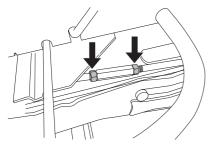
3 Screw out (extend) the stay to raise the rear edge of the cover.
