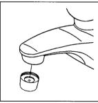
Turn on water supplies and check for leaks. With faucet off, remove aerator. Turn on hot and cold water to flush lines and faucet. Turn off faucet and replace aerator.
