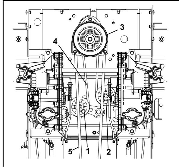
1. Spring loaded idler pulley
