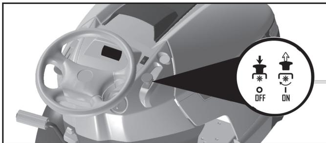
(☒) ATTACHMENT CLUTCH SWITCH "DISENGAGED"
