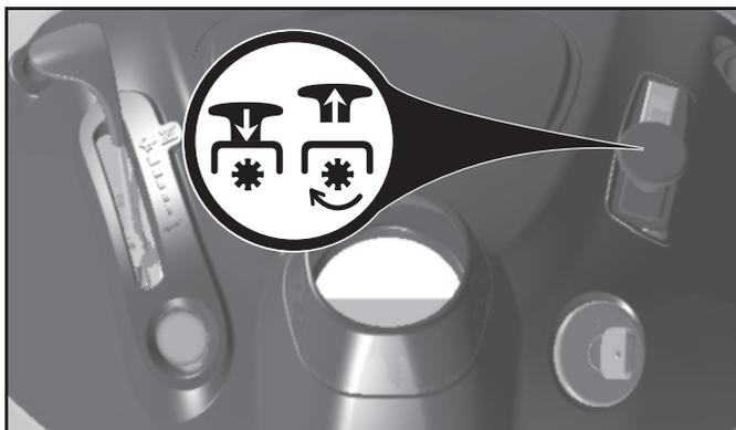
(⚙️) ATTACHMENT CLUTCH SWITCH "DISENGAGED"
