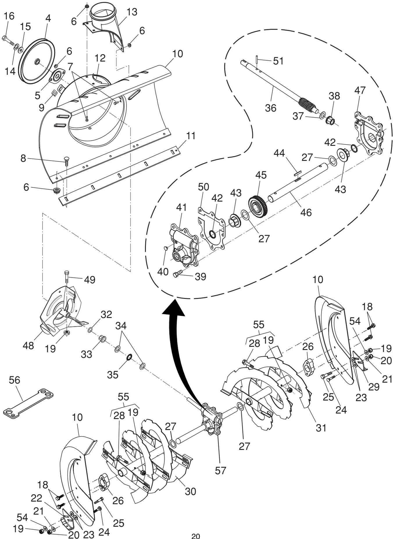
**REPAIR PARTS****AUGER HOUSING / IMPELLER ASSEMBLY****SNOW THROWER - MODEL NO. 5224SE (96193000200), PRODUCT NO. 961 93 00-02**
