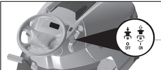
(☒) ATTACHMENT CLUTCH SWITCH "DISENGAGED"
