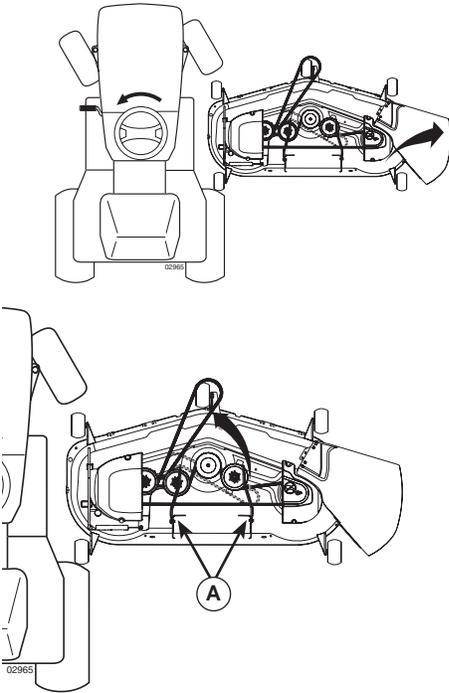
**NOTE:** Be sure mower side suspension arms (A) are pointing forward before sliding mower under tractor.
