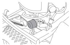
Lightly lubricate the rubber seal on the new oil filter using new oil. Fit the oil filter by turning clockwise. Turn by hand until the rubber seal is seated. Now tighten a further half turn.
