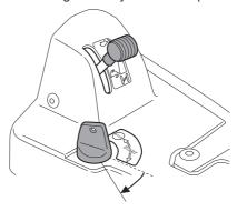
5 When the engine starts release the ignition key immediately back to neutral position.
