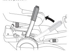
2 Move the throttle control to the MIN. position. Turn the ignition key to the "STOP".
