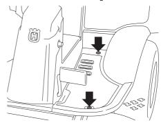
2 Loosen the locking nuts (1).
