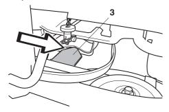
3 Insert the bolt and secure it with a locking pin.
