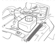
**Rider 175** Fill if necessary with engine oil SAE 10W/30 (class SF–CC).
