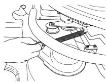
6 Place a foot on the front edge of the cutting unit near the wheel and raise the front edge of the unit to make it easier to remove the lift strut.
