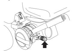
It is important that the air pressure in both front wheels is equal, 60 kPa / 8.5 PSI, to produce an even cutting height.
