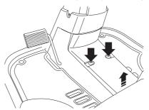
2 Check the tension of the steering wires by squeezing them together by the arrows as illustrated. It should be possible to push them together so that the distance between them is half as much, without using unnecessary force.
