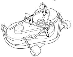
3 Loosen the spring (4) that tensions the V-belt and pry off the belt.
