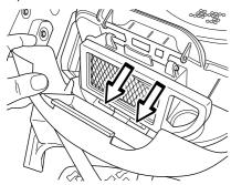
8 Pull the handle outwards. Secure the handle in the air filter cover and close the cover by pressing it inwards.
