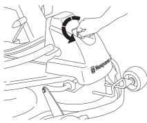
3 Remove the two support wheels from under the front hood.
