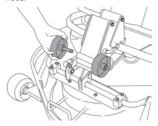
4 Fit the support wheels on either side of the rear of the cutting unit.
