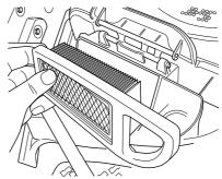
Replace the air filter cartridge, if clogged with dirt.
