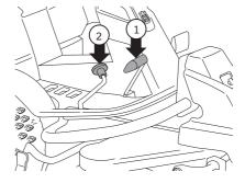
3 Select the required cutting height (1-7) with the cutting height lever.
