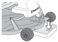
5 Adjust the unit's ground pressure by screwing in or out the adjusting screws located behind the front wheels on both sides. The ground pressure should be between 12 and 15 kg (26.5-33 lb).
