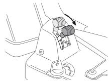
7 Set the required engine speed with the throttle control.
