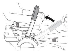
Rider 175 AWD The engine can not be started if the parking brake is not pressed down.
