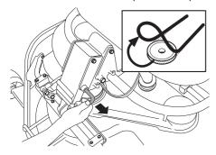
9 Pull the frame forwards and refit the pin.
