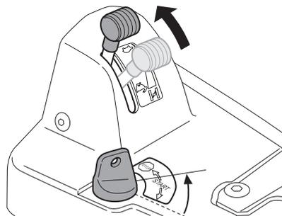
**For Rider 13 C, Rider 16 AWD and Rider 16 C** Pull back the throttle and turn the ignition key to the "STOP" position.
