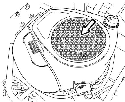
Check the air duct, located on the inside of the engine cover, ensure it is clean and does not rub against the cooling air intake.
