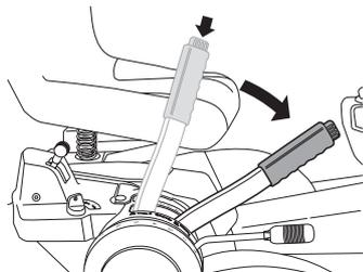
The lever can also be used to temporarily regulate the cutting height, e.g. for a small mound in the lawn.
