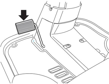
The blade drive is not affected by the clutch pedal.
