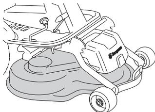
The Combi-unit, equipped with a Mulching-plug, finely chops the cuttings to fertiliser. Without the Mulching-plug the unit works in the same way as a rear ejection unit.
