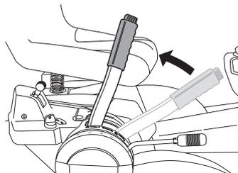
If the lock button is pressed in and the lever is moved forwards the unit will be lowered and the blades will automatically start to rotate (mowing position).
