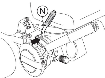
The lock button on the gear shift lever must be held in to engage reverse gear.
