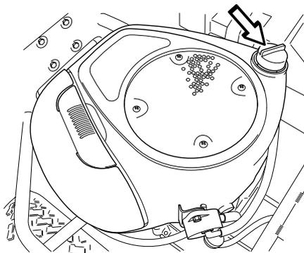
The dipstick should be **completely screwed down**
