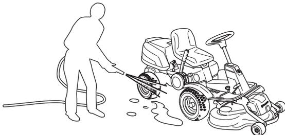
Oily dirt can be removed using a cold degreasing agent. Spray on a thin layer.
