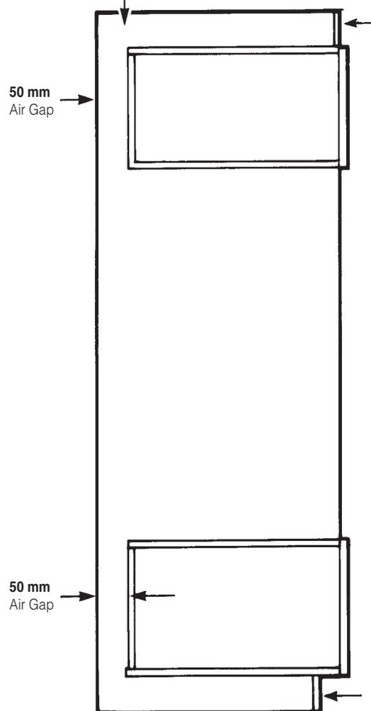
Ventilation Slot required here if the cabinet does not fit to the ceiling - 51mm x 457mm min. area
