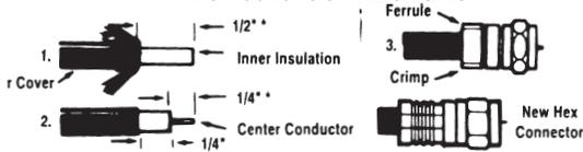
**STEP 1:** Strip outer cover back 1/2" from end of cable. Fray braid back as far as outer cover will allow.
