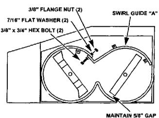
13. Scribe or pencil a mark at the locations for drilling the holes for swirl guide A. Some mower decks have pilot holes and will not require scribing.
