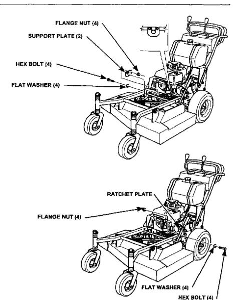
Remove the front bolt, washer and nut from the height adjustment ratchet plate.
